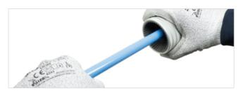
Always deburr the pipe, externally and internally, eliminating sharp edges, before making the connection with the fittings. Use the FPUS accessory.
