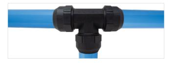
It is recommended to provide one or more drainage points for any condensation. The drainage points must be made at the lowest points of the main pipeline by using Tee fittings.
