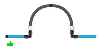
This is the correct application of the installation of expansion joint. It should be facing up and with two elbows aligned. You need also to insert two clips on the pipe aluminum fasteners close to the installation of an expansion joint.
