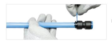
Remove the light blue locking clip by pulling it from the tab.
