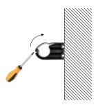
The F-Line.PRO wall fastener can be used both in horizontal or vertical position. Place the FPST at the desired height and open the hook with a screwdriver.
