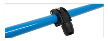
Fix the branch so that the internal part will stay correctly in the hole. F-Line.PRO branches have a guided air intake that go inside the tube so that, once they are fixed, it will be impossible for them to move from their position. This system ensure the functioning, always guaranteeing the maximum air flow and eliminating any risk of leakages.
