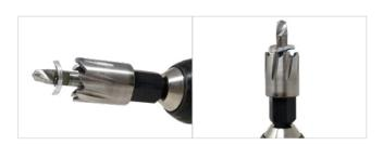
Position the mill vertically, allowing the hook to fall inside the outline of the tip and remove the residual aluminum disk.
