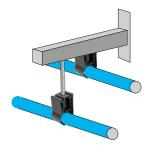
You can secure the wall fastener to any type of clamping system and then insert the tube into the wall fastener and set the hook.
