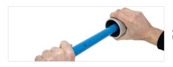
Always deburr the tubes and brake sharp edges before connecting them with F-Line.PRO fittings using FPUS beveling cone.
