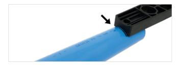
Mark the tube using the back part of the proper spanner in order to identify the correct and full insertion of the tube after installation.
