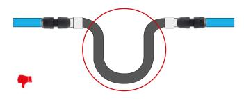
Always install the expansion joint facing upwards and not downwards in order to avoid a deposit of the condensation.
