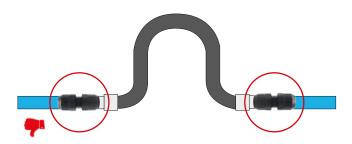
Avoid anchoring the expansion joint to two connections aligned to the same plan.
