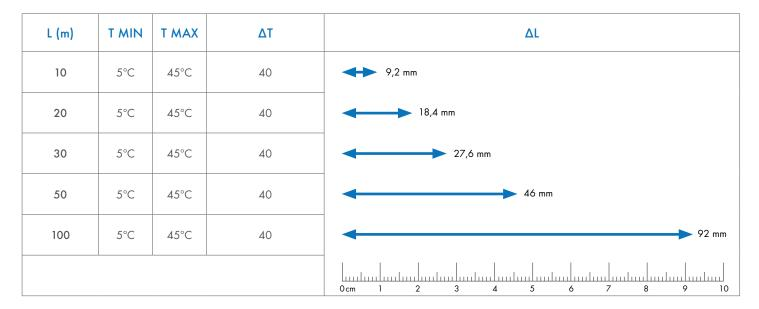
Table of contraction - expansion depending on the length L of a straight stretch and the temperature difference  $\Delta T$ .
